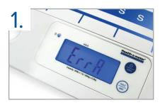
While preparing to weigh a patient, ensure there are no more than 8" between each stretcher/bed or stretcher/stretcher. The scale should not be tilted and must be as level as possible. The PTS has an electronic level and if the scale is not flat an "ERR A" message will appear. If the "ERR A" code does appear, do not remove the patient from the scale, just lower one surface until level and the weight comes up.
