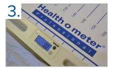
Lay the Patient Transfer scale flat onto the stretcher or bed and turn the scale on by pressing the blue power button.
