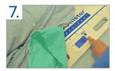
When the patient is in the middle of the scale, the accurate weight of your patient will appear on the display. If needed, a HOLD function is available. No weight recordings are stored within the PTS, however the weight will hold until the scale is moved or a button is pressed.
