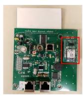
Obtain the front cover of the display head with the keypad removed in step 3. Plug the keypad cable into its port on the PCB.
