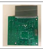
6. Obtain the green wireless module from the packaging. Carefully insert the wireless module into the Port JR1 on the back of the PCB as shown. Observe the orientation of the wireless module. Gently press until secure, do not apply extreme pressure.
