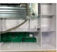
6. Carefully replace the metal plate and replace the 3 screws obtained in step 3, and reinstall the batteries.
