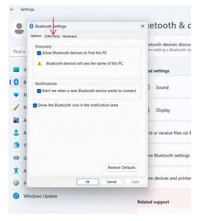
12. In the COM Ports tab, note down the COM Port Number shown next to the HOM Scale "Outgoing". Use this COM Port "COM#" to communicate with the scale wirelessly to transfer data (COM11 in this image).
