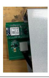
6. Carefully close the display head and replace the 4 screws obtained in step 3, and reinstall the batteries.
