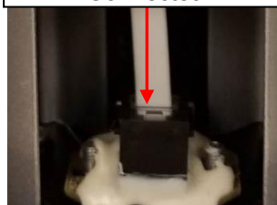
Load Cell Cable Connected
