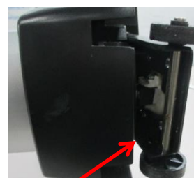
Gap at Rear of Platform
