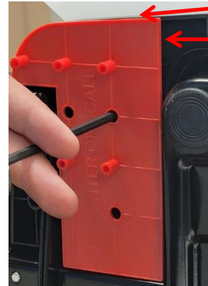
Align edge of drill guide with edge of scale platform
