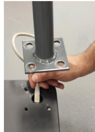
3. Holding the handrail in place, tip the platform forward to be able to access the underside of the platform. Pull the cable through the ring shaped hole behind the wheel then feed the cable through the metal shield as shown.
