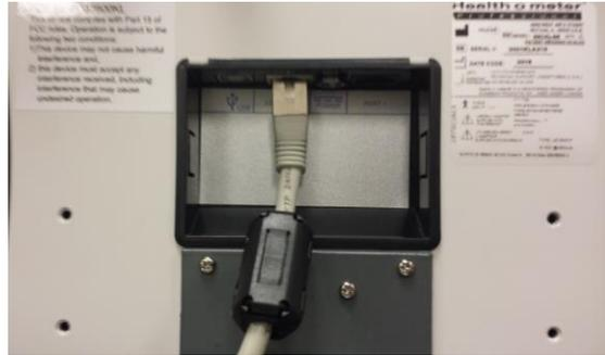
8. Attach the adapter holder to the handrail using the (2) included sheet metal screws. Use a Phillips head screwdriver to tighten the screws. The scale is now assembled. See Powering the Scale on page 10 for battery/AC adapter instructions.
