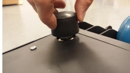
2. Turn the platform over so it is facing up. Locate the handrail and untie the load cell cable connector. Position the handrail over the handrail supports on the platform and feed the cable through the ring shaped hole located on the right handrail support.
