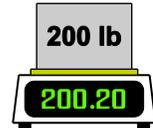
The **accuracy** of a scale is a measure of the degree of closeness of the average value of an object's displayed weight to the object's actual weight. If, on average, a scale indicates that a 200 lb reference weight weighs 200.20 lb, then the scale is accurate to within 0.20 lb in 200 lb, or 0.1%.
